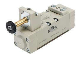
NITRA solenoid valve, ISO 5599/1 size 1, 5-way, 2-position, single solenoid spring return, aluminum alloy body, locking manual override.
