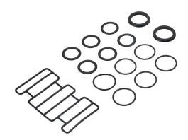
NITRA seal kit, replacement. For use with ISO 5599/1 size 2 solenoid valves. Includes o-rings, lip seals and valve bottom gasket.
