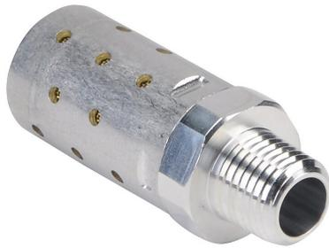
NITRA pneumatic exhaust silencer, aluminum, cylindrical, Cv=2.7, 1/4in male NPT.
