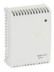
ProSense temperature/humidity sensor, room sensor, plastic wall mounting subplate process connection, Output: 2-channel, current, -19.9 to +60  $^{\circ}$ C, 0 to 99.9% RH, IP10, wall mount, screw terminals.
