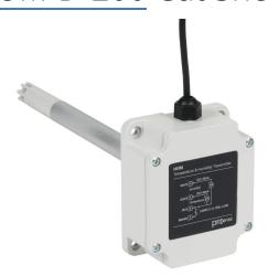
ProSense temperature/humidity sensor, duct insertion probe, 200mm insertion length, Output: 2-channel, current, -19.9 to +60 °C, 0 to 99.9% RH, duct mount, 6.5ft/2m 22 AWG wire leads.
