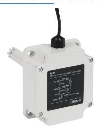
ProSense temperature/humidity sensor, duct insertion probe, 100mm insertion length, Output: 2-channel, current, -19.9 to +60 °C, 0 to 99.9% RH, duct mount, 6.5ft/2m 22 AWG wire leads.
