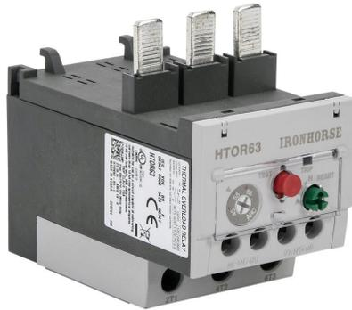
IronHorse thermal overload relay, 45-65A adjustable, bi-metallic, direct mount power connection(s). For use with HMC-50 and HMC-65 Contactors.
