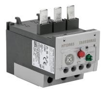
IronHorse thermal overload relay, 34-50A adjustable, bi-metallic, direct mount power connection(s). For use with HMC-50 and HMC-65 Contactors.
