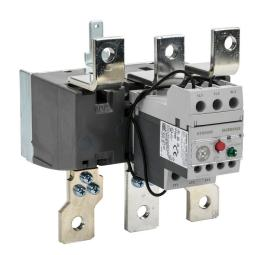
IronHorse thermal overload relay, 200-330A adjustable, bimetallic, direct mount power connection(s). For use with HMC-265 to HMC-400 contactors.
