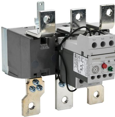
IronHorse thermal overload relay, 160-240A adjustable, bi-metallic, direct mount power connection(s). For use with HMC-265 to HMC-400 contactors.
