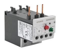
IronHorse thermal overload relay, 5-8A adjustable, bi-metallic, direct mount power connection(s). For use with HMC-9 to HMC-40 contactors.
