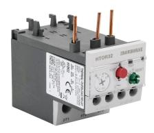
IronHorse thermal overload relay, 28-40A adjustable, bi-metallic, direct mount power connection(s). For use with HMC-9 to HMC-40 contactors.
