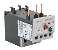
IronHorse thermal overload relay, 2.5-4A adjustable, bi-metallic, direct mount power connection(s). For use with HMC-9 to HMC-40 contactors.
