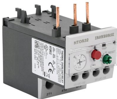
IronHorse thermal overload relay, 12-18A adjustable, bi-metallic, direct mount power connection(s). For use with HMC-9 to HMC-40 contactors.
