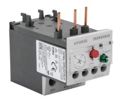
IronHorse thermal overload relay, 7-10A adjustable, bi-metallic, direct mount power connection(s). For use with HMC-9 to HMC-40 contactors.
