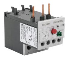
IronHorse thermal overload relay, 0.25-0.40A adjustable, bimetallic, direct mount power connection(s). For use with HMC-9 to HMC-40 contactors.
