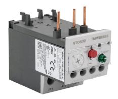
IronHorse thermal overload relay, 0.10-0.16A adjustable, bimetallic, direct mount power connection(s). For use with HMC-9 to HMC-40 contactors.
