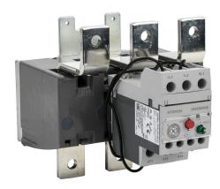
IronHorse thermal overload relay, 120-185A adjustable, bimetallic, direct mount power connection(s). For use with HMC-185 and HMC-225 contactors.
