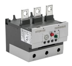
IronHorse thermal overload relay, 110-150A adjustable, bimetallic, direct mount power connection(s). For use with HMC-130 and HMC-150 contactors.
