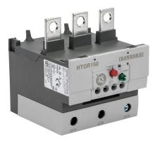
IronHorse thermal overload relay, 80-105A adjustable, bi-metallic, direct mount power connection(s). For use with HMC-130 and HMC-150 contactors.
