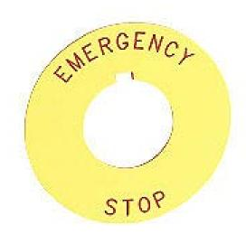
Eaton legend plate, plastic, round, yellow field, yellow background, red engraved text, legend plate marking "EMERGENCY STOP". For use with 30mm pilot devices.
