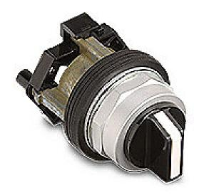
Eaton selector switch, 30mm, 3-position, spring return to center, operator only, metal base, metal bezel, Operator: black, knob, 27mm, round, plastic.
