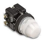
Eaton incandescent indicating light, permanent light function, 30mm, white, 32mm, round, metal base, metal bezel, 24 VAC/ VDC, full voltage.
