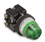
Eaton incandescent indicating light, permanent light function, 30mm, green, 32mm, round, metal base, metal bezel, 120 VAC/VDC, full voltage.
