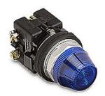
Eaton incandescent indicating light, permanent light function, 30mm, blue, 32mm, round, metal base, metal bezel, 120 VAC/VDC, full voltage.
