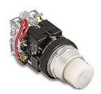
Eaton incandescent indicating light, permanent light function, 30mm, push-to-test, white, 32mm, round, metal base, metal bezel, 120 VAC/VDC, full voltage.
