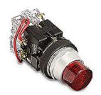
Eaton incandescent indicating light, permanent light function, 30mm, push-to-test, red, 32mm, round, metal base, metal bezel, 120 VAC/VDC, full voltage.
