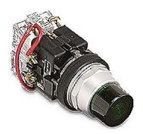
Eaton incandescent indicating light, permanent light function, 30mm, push-to-test, green, 32mm, round, metal base, metal bezel, 120 VAC/VDC, full voltage.
