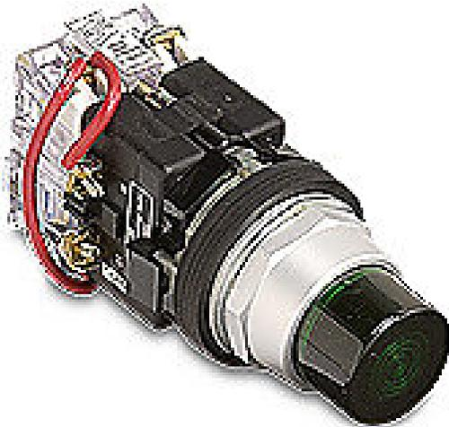
Eaton incandescent indicating light, permanent light function, 30mm, push-to-test, green, 32mm, round, metal base, metal bezel, 24 VAC/VDC, full voltage.
