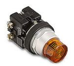
Eaton incandescent indicating light, permanent light function, 30mm, push-to-test, amber, 32mm, round, metal base, metal bezel, 24 VAC/VDC, full voltage.
