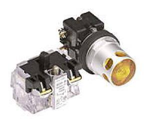
Eaton pushbutton, 30mm, momentary, incandescent illuminated, (1) N.C. contact(s), metal base, metal bezel, guarded, Operator: yellow, flush, 28mm, round, plastic, 24 VAC/VDC, full voltage.
