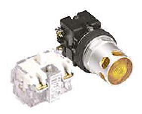
Eaton pushbutton, 30mm, momentary, incandescent illuminated, (1) N.O. contact(s), metal base, metal bezel, guarded, Operator: yellow, flush, 28mm, round, plastic, 24 VAC/VDC, full voltage.
