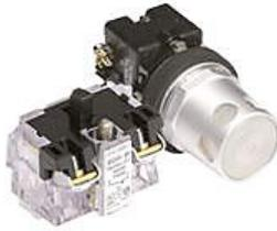
Eaton pushbutton, 30mm, momentary, incandescent illuminated, (1) N.C. contact(s), metal base, metal bezel, guarded, Operator: white, flush, 28mm, round, plastic, 24 VAC/VDC, full voltage.
