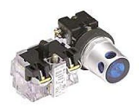
Eaton pushbutton, 30mm, momentary, incandescent illuminated, (1) N.C. contact(s), metal base, metal bezel, guarded, Operator: blue, flush, 28mm, round, plastic, 24 VAC/VDC, full voltage.
