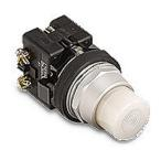
Eaton pushbutton, 30mm, momentary, incandescent illuminated, operator only, metal base, metal bezel, Operator: white, extended, 28mm, round, plastic, 24 VAC/VDC, full voltage.
