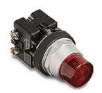
Eaton pushbutton, 30mm, momentary, incandescent illuminated, operator only, metal base, metal bezel, Operator: red, extended, 28mm, round, plastic, 120 VAC/VDC, full voltage.
