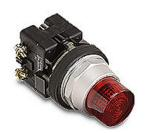
Eaton pushbutton, 30mm, momentary, incandescent illuminated, operator only, metal base, metal bezel, Operator: red, extended, 28mm, round, plastic, 24 VAC/VDC, full voltage.
