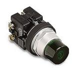
Eaton pushbutton, 30mm, momentary, incandescent illuminated, operator only, metal base, metal bezel, Operator: green, extended, 28mm, round, plastic, 24 VAC/VDC, full voltage.
