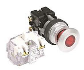
Eaton pushbutton, 30mm, push to lock, pull to reset, incandescent illuminated, (1) N.O. contact(s), metal base, metal bezel, Operator: red, mushroom, 42mm, round, plastic, 24 VAC/VDC, full voltage.
