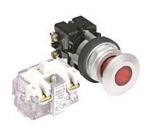
Eaton pushbutton, 30mm, push to lock, pull to reset, LED illuminated, (1) N.O. contact(s), metal base, metal bezel, Operator: red, mushroom, 42mm, round, plastic, 24 VAC/VDC, full voltage.
