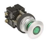
Eaton pushbutton, 30mm, push to lock, pull to reset, incandescent illuminated, operator only, metal base, metal bezel, Operator: green, mushroom, 42mm, round, plastic, 24 VAC/VDC, full voltage.
