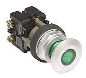
Eaton pushbutton, 30mm, push to lock, pull to reset, incandescent illuminated, operator only, metal base, metal bezel, Operator: green, mushroom, 42mm, round, plastic, 24 VAC/VDC, full voltage.
