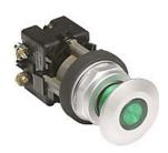
Eaton pushbutton, 30mm, push to lock, pull to reset, LED illuminated, operator only, metal base, metal bezel, Operator: green, mushroom, 42mm, round, plastic, 24 VAC/VDC, full voltage.
