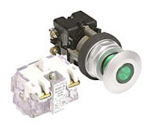
Eaton pushbutton, 30mm, push to lock, pull to reset, incandescent illuminated, (1) N.O. contact(s), metal base, metal bezel, Operator: green, mushroom, 42mm, round, plastic, 24 VAC/VDC, full voltage.
