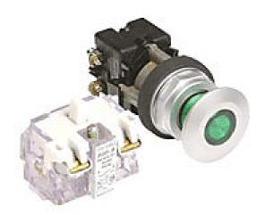
Eaton pushbutton, 30mm, push to lock, pull to reset, LED illuminated, (1) N.O. contact(s), metal base, metal bezel, Operator: green, mushroom, 42mm, round, plastic, 24 VAC/VDC, full voltage.
