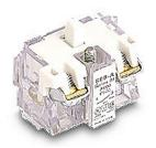
Eaton contact block, replacement, 30mm, (1) N.O. contact(s), gold-plated. For use with HT800 series pushbuttons and switches.
