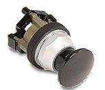
Eaton pushbutton, 30mm, momentary, operator only, metal base, metal bezel, Operator: black, mushroom, 40mm, round, plastic.
