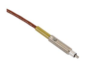
Metrol limit switch, high temperature, precision touch, 6mm diameter, threaded, 0.75mm pitch, 45.5mm length, 1.5mm radius head, 2mm plunger, 1N contact force, N.O. contact(s), 6.5ft/2m cable length, pigtail.
