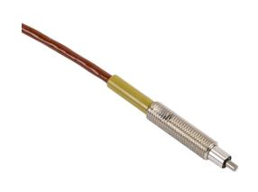
Metrol limit switch, high temperature, precision touch, 6mm diameter, threaded, 0.75mm pitch, 45.5mm length, 1.5mm radius head, stainless steel, 2mm plunger, 1N contact force, (1) N.O. contact(s), 6.5ft/2m cable length, pigtail.
