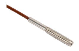
Metrol limit switch, high temperature, precision touch, 6mm diameter, threaded, 1mm pitch, 47.8mm length, 3mm head, stainless steel, ball plunger, 6-13N contact force, (1) N.O. contact(s), 6.5ft/2m cable length, pigtail.
