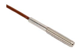
Metrol limit switch, high temperature, precision touch, 6mm diameter, threaded, 1mm pitch, 47.8mm length, 3mm head, ball plunger, 6-13N contact force, N.O. contact(s), 6.5ft/2m cable length, pigtail.
