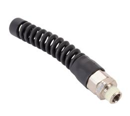
NITRA pneumatic or water threaded fitting, male, hose rigid, nickel-plated brass body, nickel-plated brass threads, thread sealant, 3/8in inside diameter to 3/8in male NPT.
