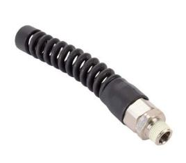
NITRA air or water threaded fitting, male, hose rigid, nickel-plated brass body, nickel-plated brass threads, thread sealant, 3/8in inside diameter to 3/8in male NPT.
