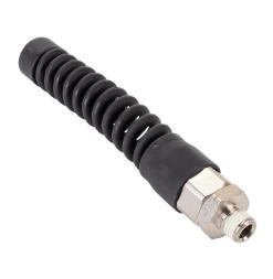
NITRA pneumatic or water threaded fitting, male, hose rigid, nickel-plated brass body, nickel-plated brass threads, thread sealant, 3/8in inside diameter to 1/4in male NPT.
